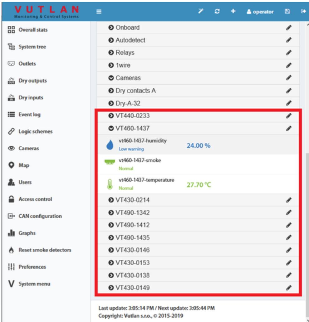
If after clicking the "Configure" button the poll is reset to the phrase "Update", then the line is not connected or the terminators on the bus are not agreed. It is necessary to check and change the condition of the **TR terminators** (See "TR termination switch" section above) on the modules or check and possibly change the **connection cables**.
