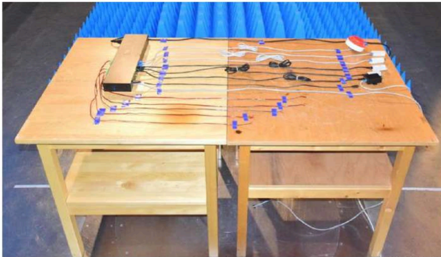
Fig.5: Arrangement of tested sample during the test according to EN 61000-4-3.
