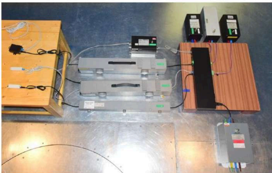
Fig.7: Arrangement of tested sample during the test according to EN 61000-4-6.
