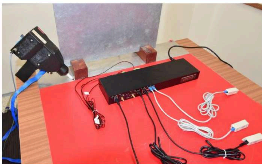
Fig.4: Arrangement of tested sample during the test according to EN 61000-4-2.
